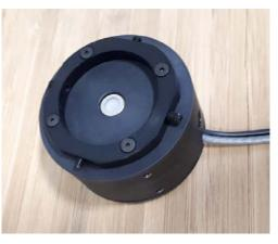
The spectral range is limited by high density polyethylene window.
